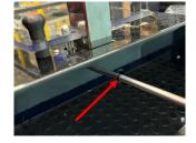
After positioning the supplied tube, tighten it slightly; the correct positioning will be done later.
